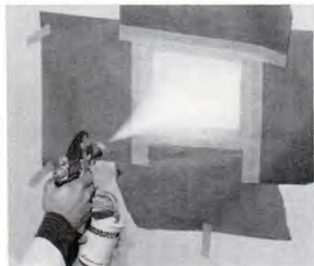
SPRAY FOR BEST OVERALL RESULTS. All you need is the spray head and compressed air. You can use a paper cup for a dispenser as demonstrated above
